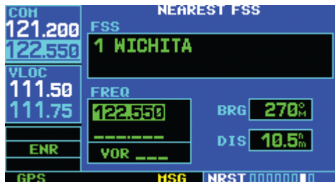
Figure 8-28 Frequency Moved to Standby Field
