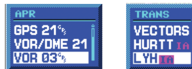
Figure 6-11 Approach and Transitions Windows
