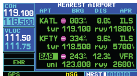
Figure 8-11 Frequency Moved to Standby Field
