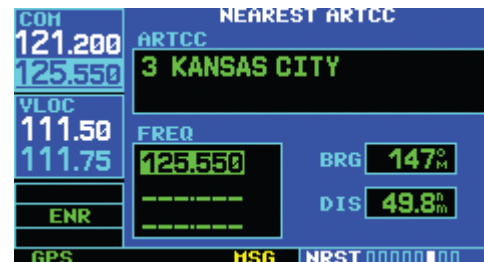
Figure 8-24 Frequency Moved to Standby Field
