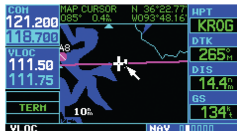
Figure 7-43 Activate Panning Function
