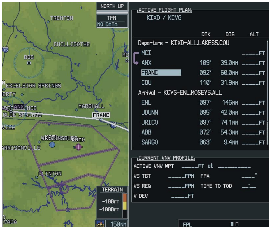
Figure 5-74 Airway Insertion Point
