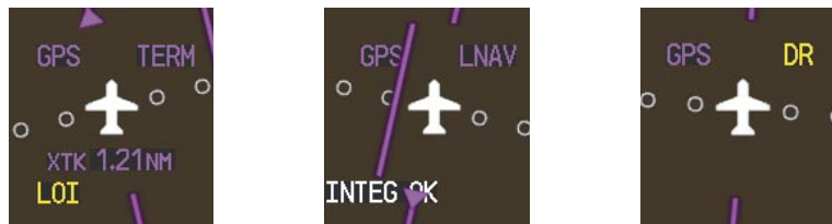
Figure 2-41 Example HSI Annunciations
