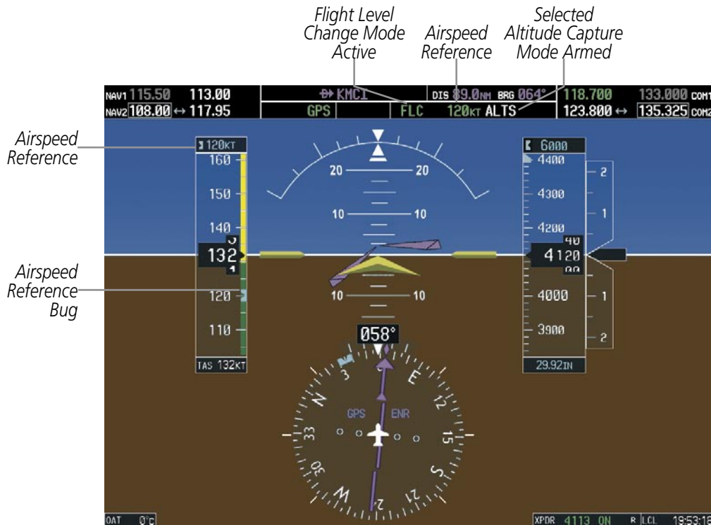
Figure 7-9 Flight Level Change Mode (IAS)
