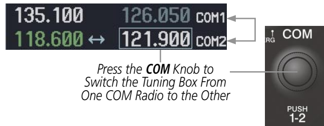
Figure 4-6 Switching COM Tuning Boxes
