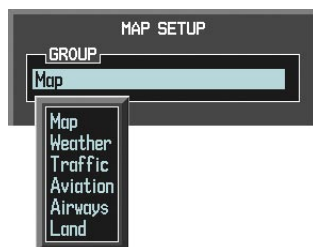
Figure 6-45 Navigation Map Page Setup Menu
