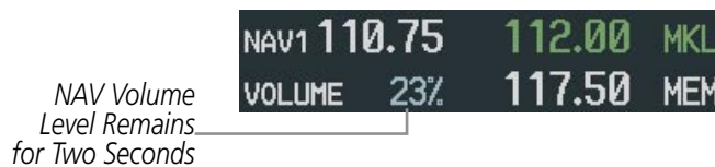
Figure 4-22 NAV Volume Levels
