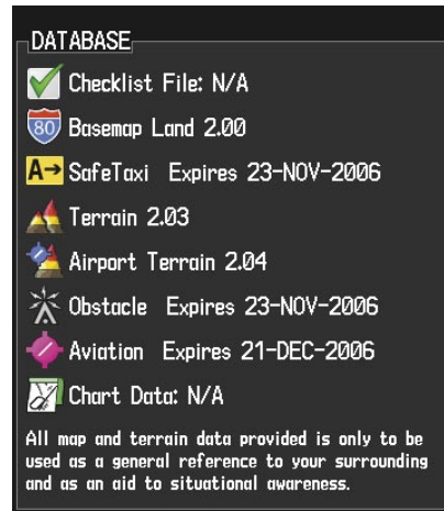
Figure B-4 Database Information on the Splash Screen
