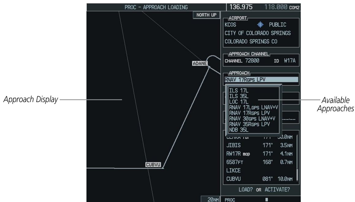
Figure 5-147 Selecting an Approach
