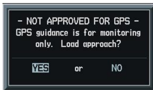
Figure 5-149 Not Approved for GPS Message
