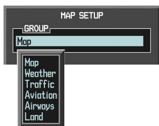
Figure 6-52 Navigation Map Page Setup Menu
