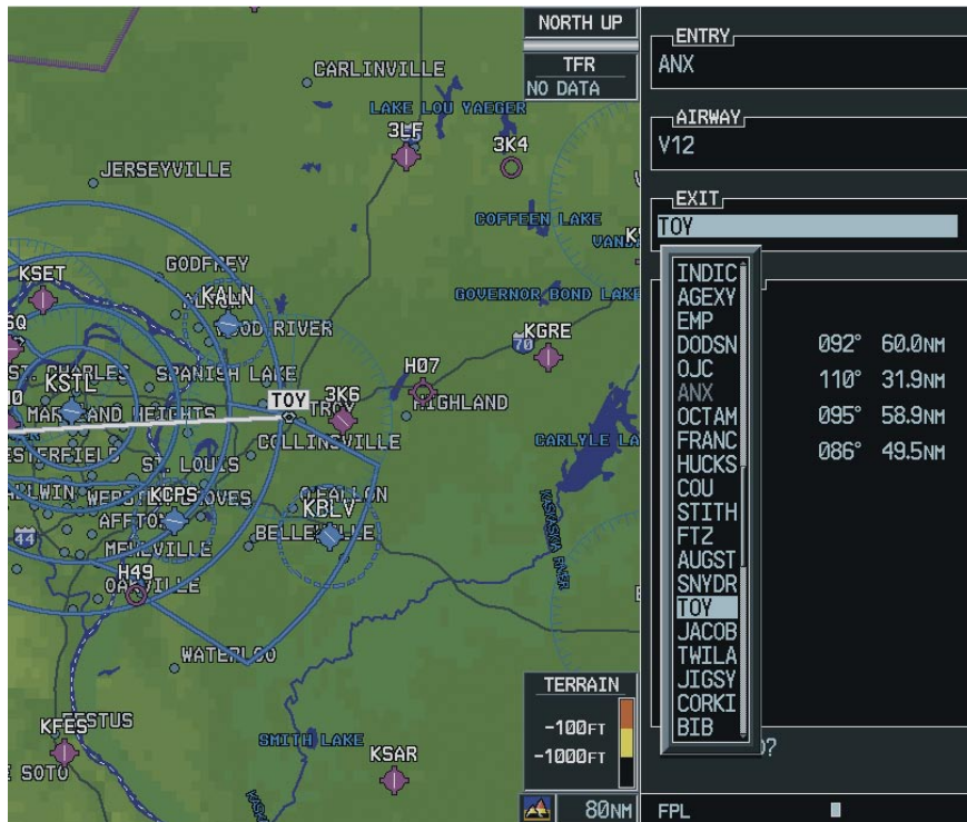
Figure 5-78 Previewing the Waypoint Sequence
