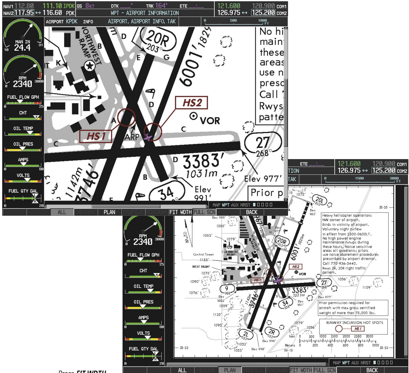
Figure 8-27 Airport Information Page, FIT WIDTH Softkey Selected
