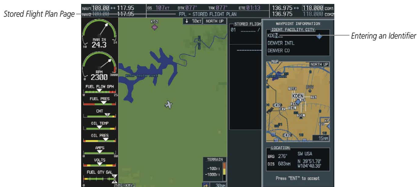
Figure 5-60 Creating a Flight Plan
