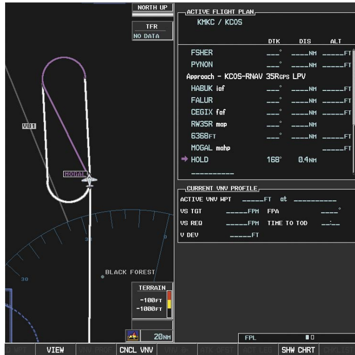
Figure 5-131 Establishing the Holding Pattern
