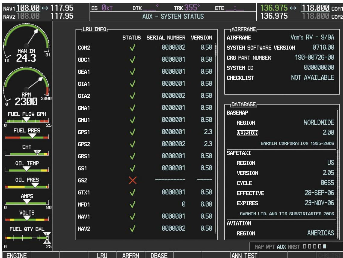
Figure 1-9 Example System Status Page
