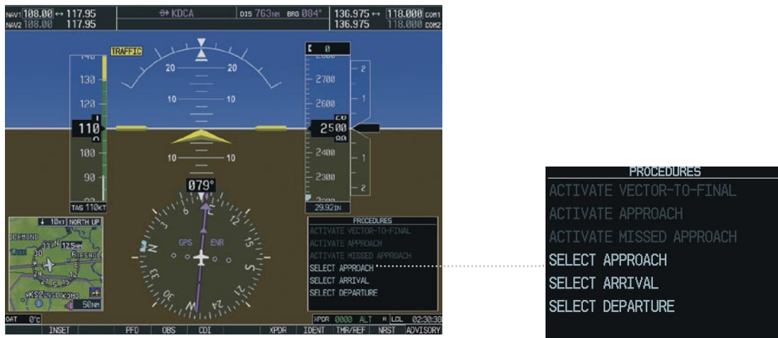
Figure 5-20 PFD Window Location
