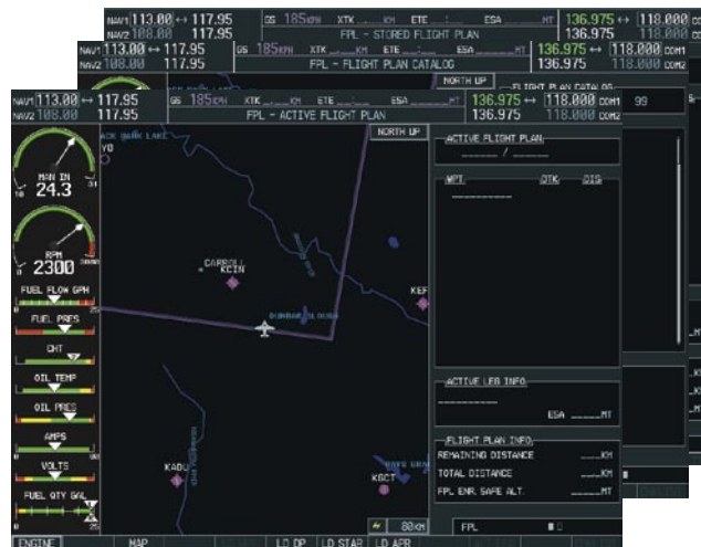
Figure 1-27 Flight Plan Pages
