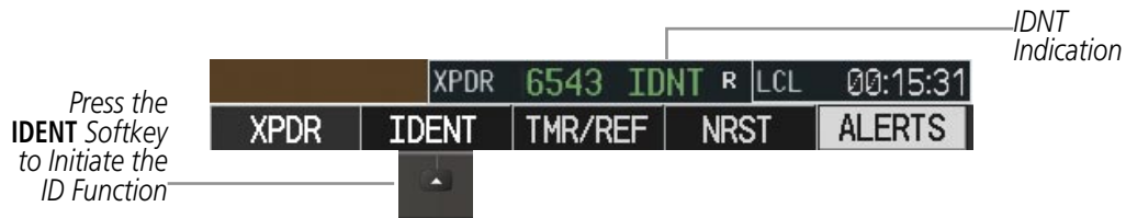
Figure 4-54 IDENT Softkey and Indication
