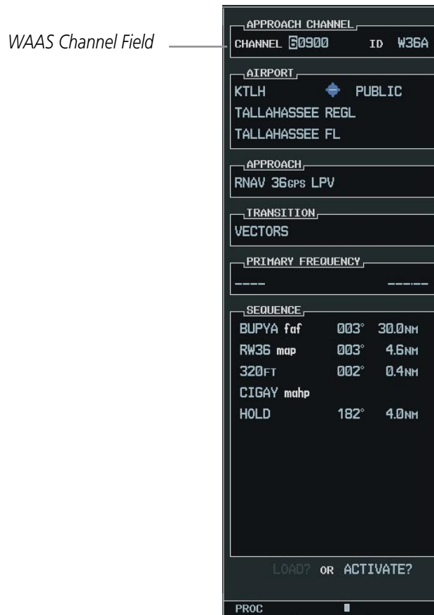
Figure 5-150 WAAS Channel Selection
