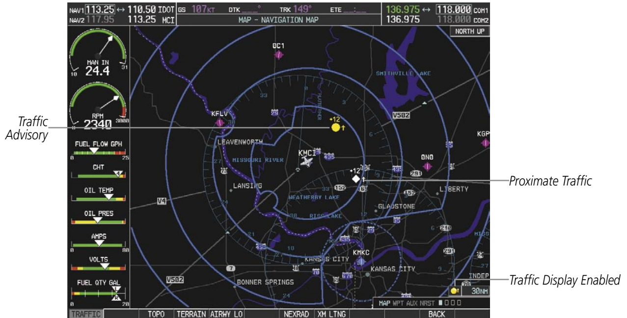
Figure 6-70 TAS Traffic on the Navigation Map Page
