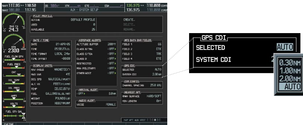
Figure 2-24 System Setup Page, GPS CDI Settings
