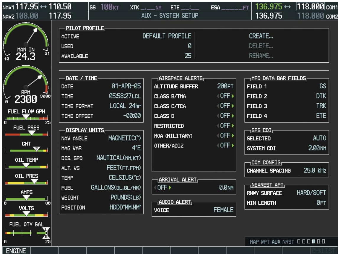
Figure 1-29 System Setup Page
