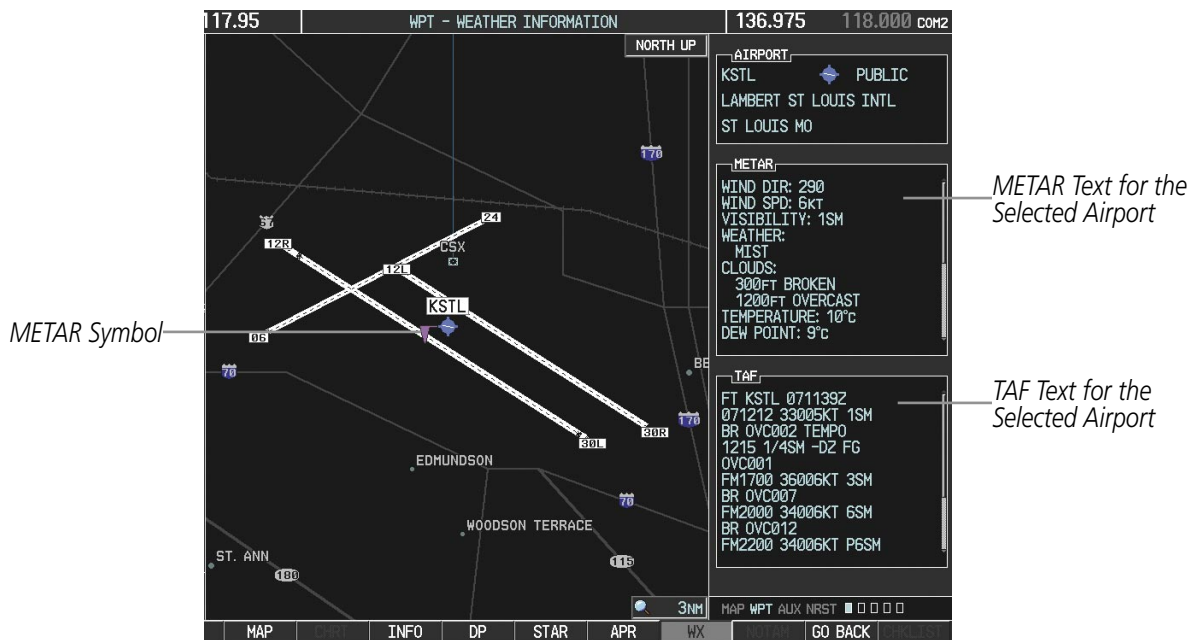
Figure 6-25 METAR and TAF Text on the Weather Information Page
