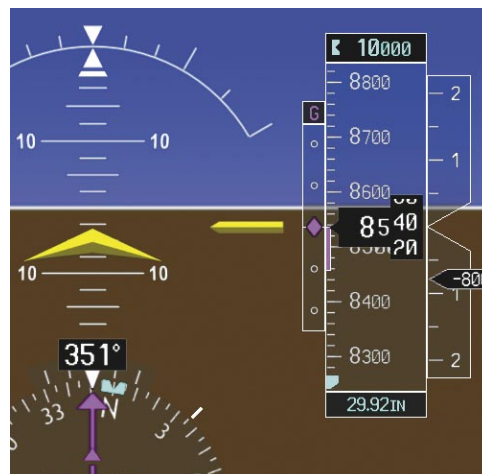
Figure 5-128 Descending to the FAF
