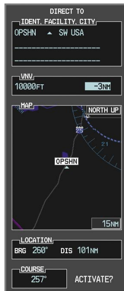
Figure 5-108 Enter VNV Offset Distance
