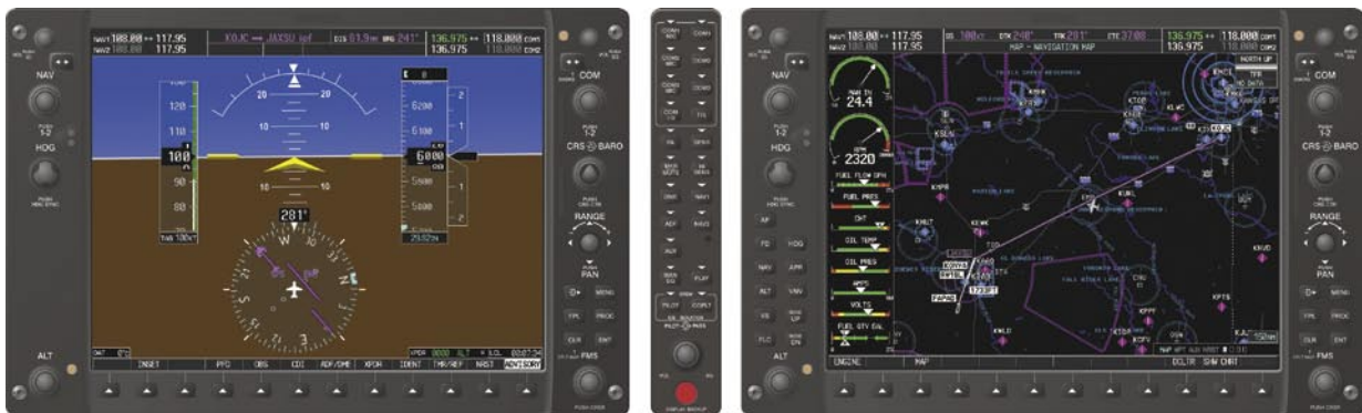
Figure 1-6 G1000 Normal Operation
