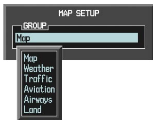
Figure 6-65 Navigation Map Page Setup Menu
