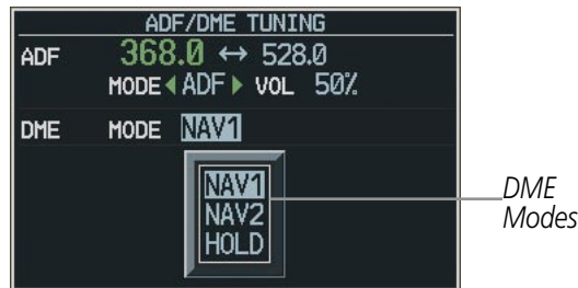
Figure 4-34 ADF/DME Tuning Window, DME Modes
