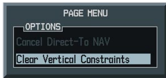
Figure 5-38 Clear Vertical Constraints Menu Option
