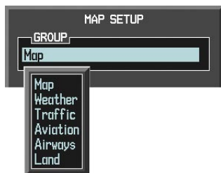
Figure 6-72 Navigation Map Page Setup Menu
