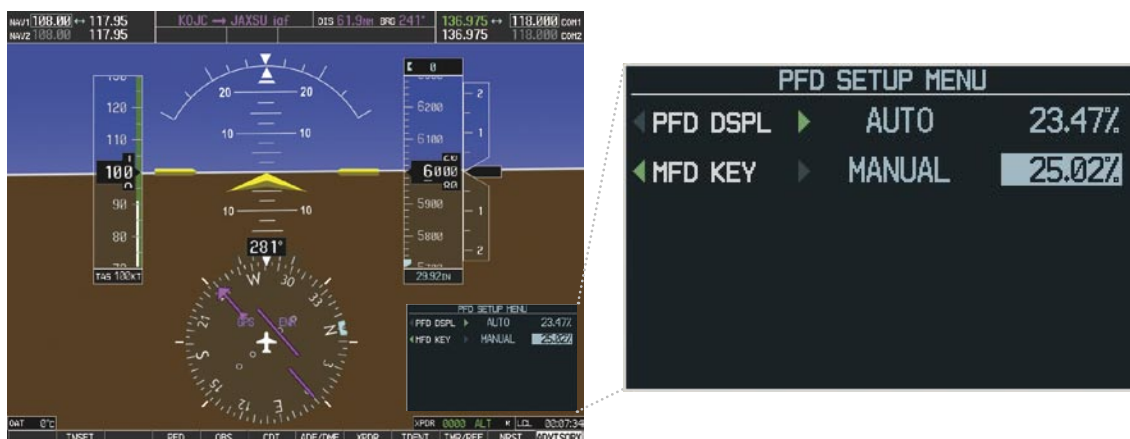
Figure 1-39 PFD Setup Menu
