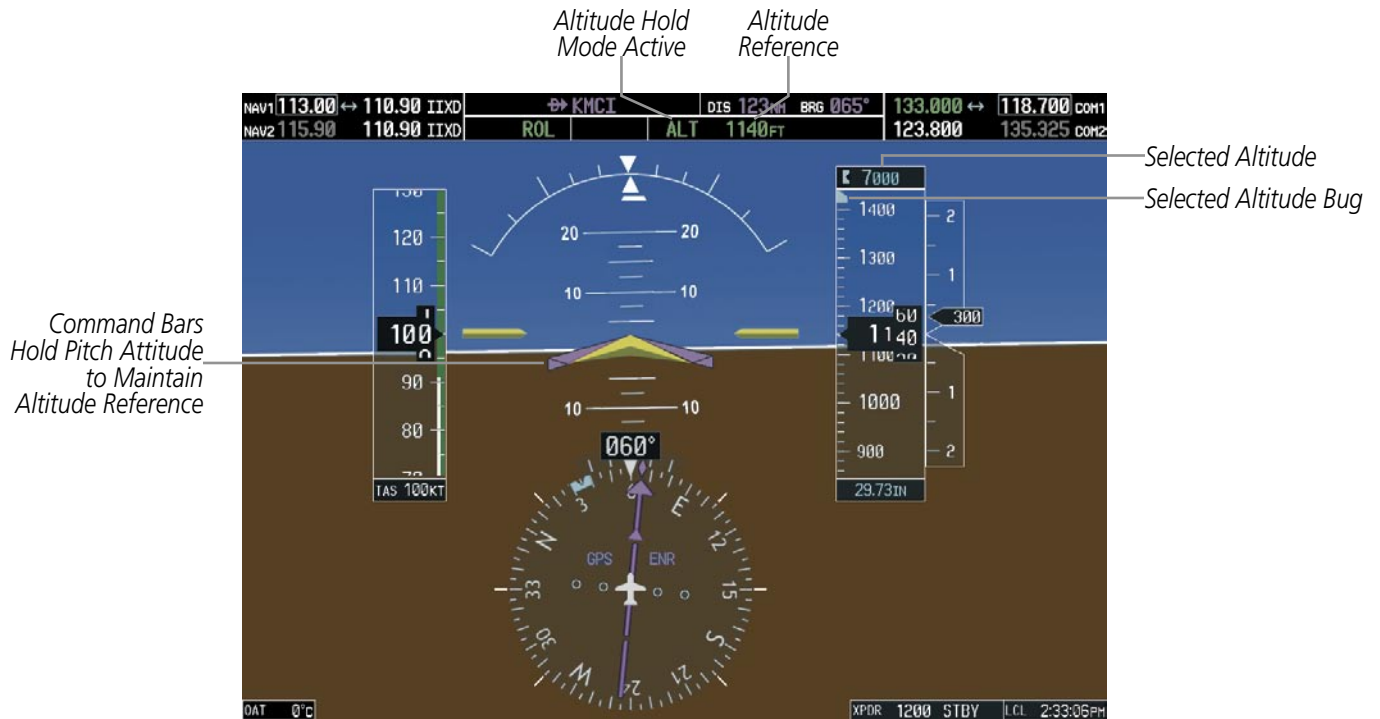
Figure 7-7 Altitude Hold Mode
