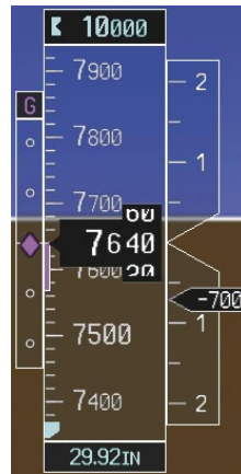
Figure 5-129 Descending to the Missed Approach Point
