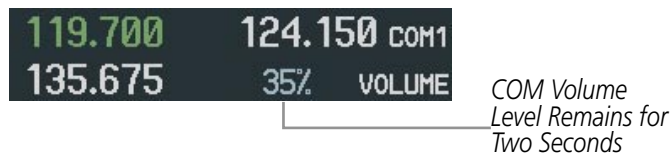
Figure 4-16 COM Volume Level
