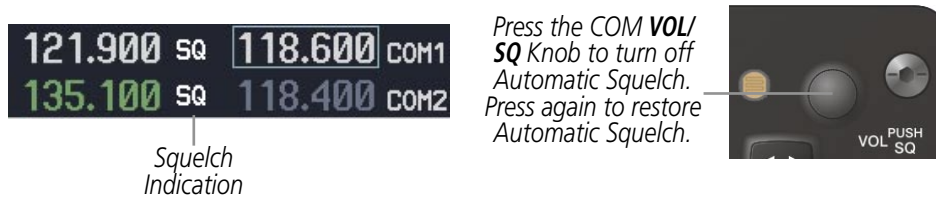
Figure 4-15 Overriding Automatic Squelch
