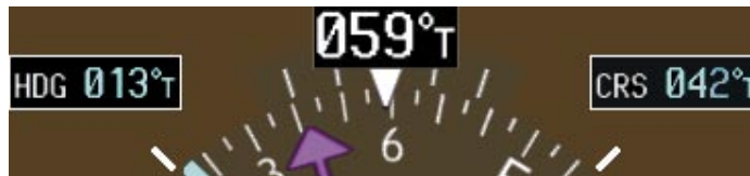
Figure 2-17 Heading and Course Indications (True)
