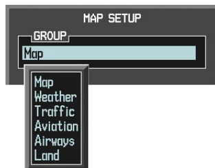
Figure 6-7 Navigation Map Page Setup Menu
