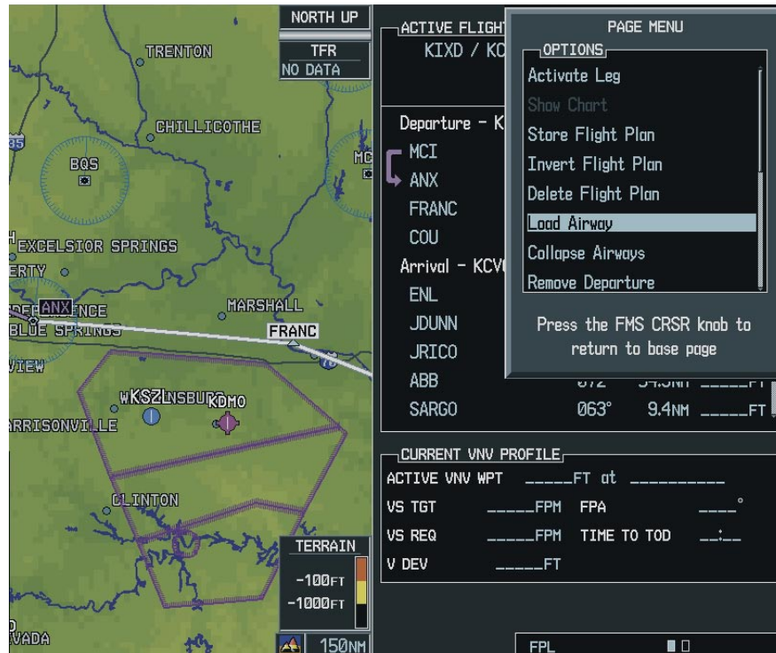
Figure 5-75 Load Airway Menu Option
