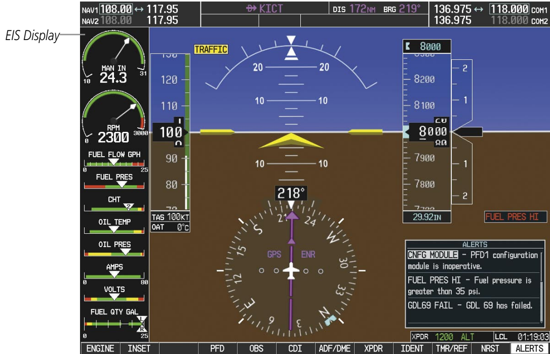
Figure 3-9 Reversionary Mode (DA40)
