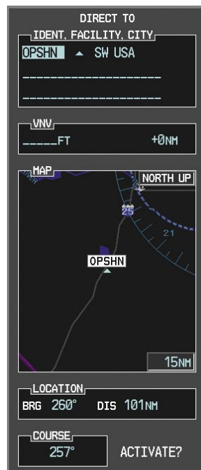
Figure 5-106 Direct To OPSHN
