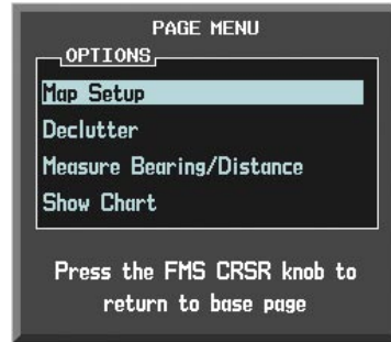
Figure 8-2 Navigation Map PAGE MENU, Map Setup Option
