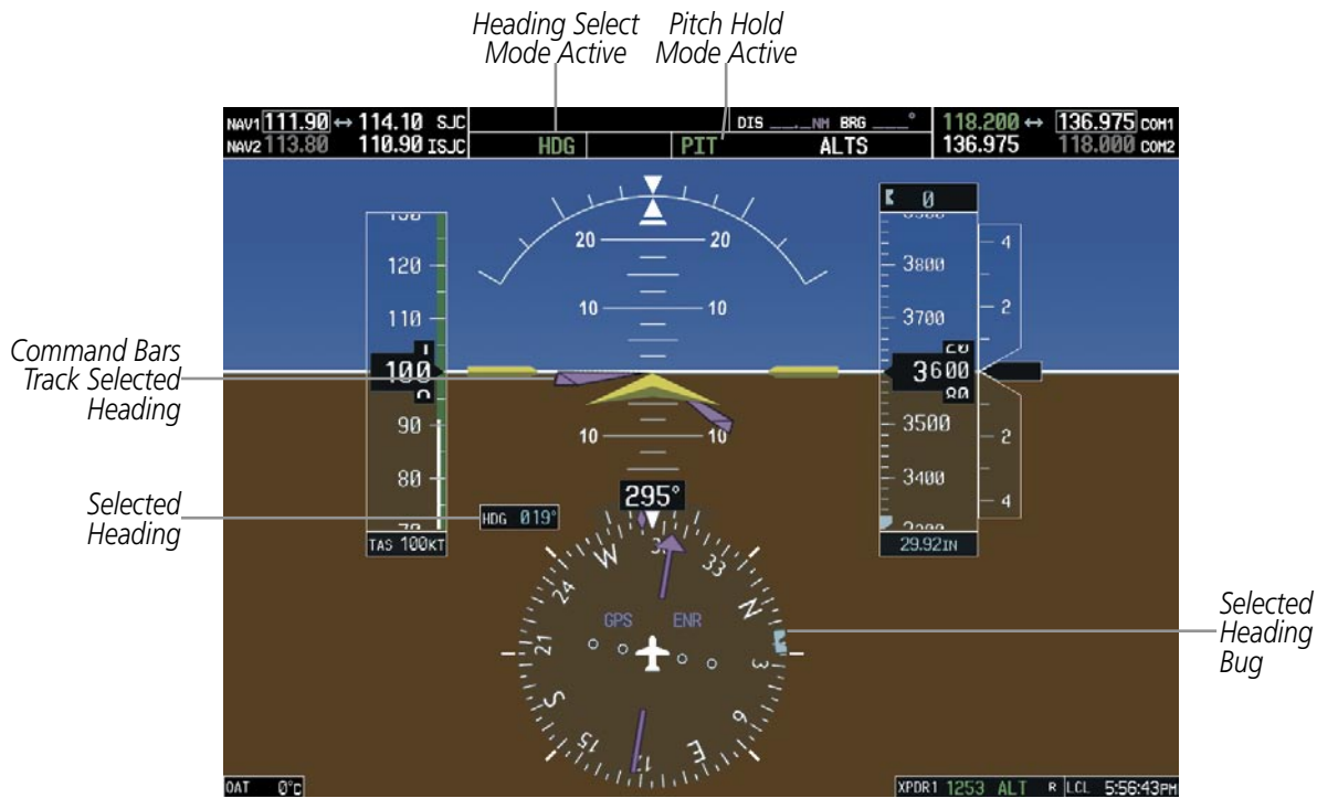
Figure 7-21 Heading Select Mode
