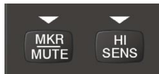
Figure 4-28 Marker Beacon Keys
