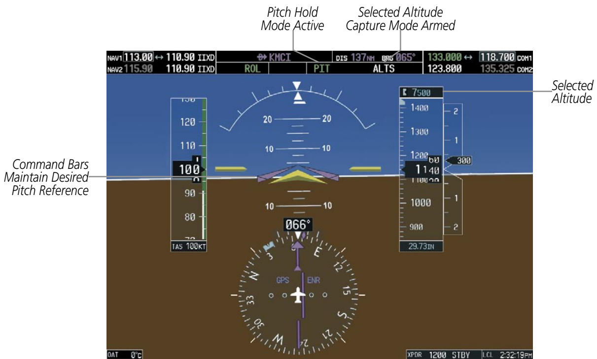
Figure 7-5 Pitch Hold Mode
