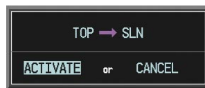
Figure 5-100 Confirm Active Leg
