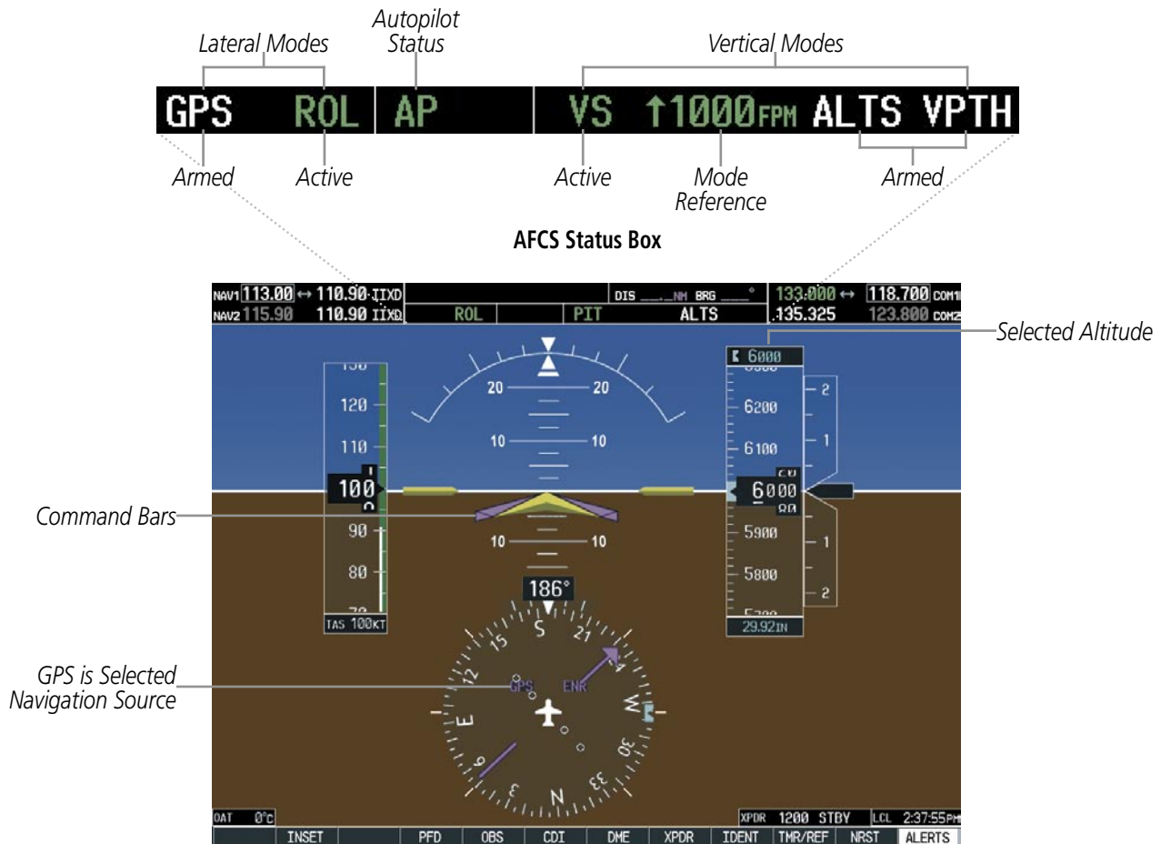
Figure 7-2 PFD AFCS Display
