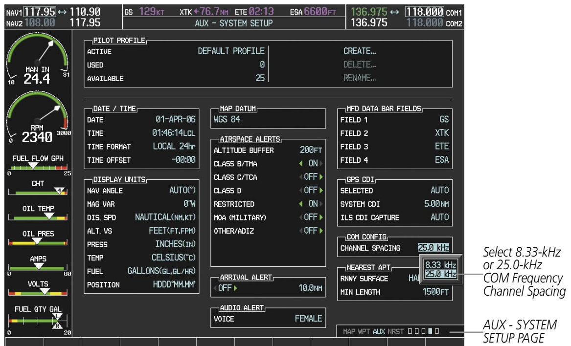
Figure 4-14 AUX – System Setup Page
