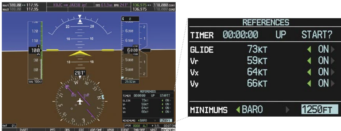
Figure 1-33 Generic Timer (Timer/References Window)
