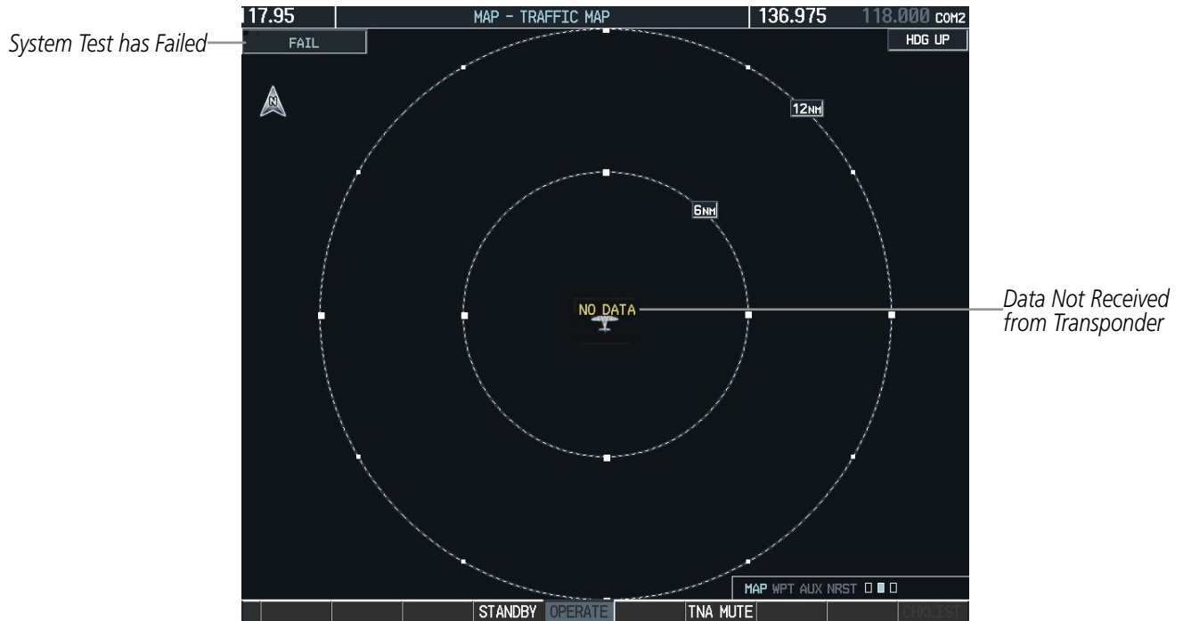
Figure 6-69 TIS Power-up Test Failure
