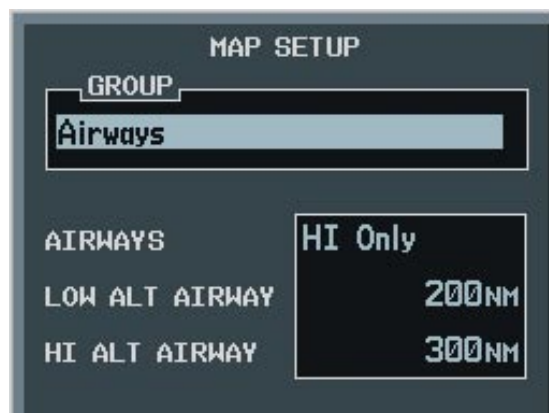
Figure 5-9 Airways Setup Options
