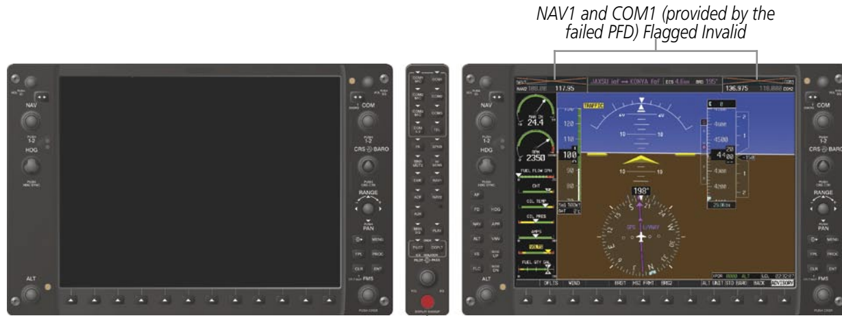
DISPLAY BACKUP Button Manually Activates/Deactivates Reversionary Mode on Both Displays
