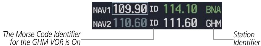
Figure 4-21 NAV Radio ID Indication
