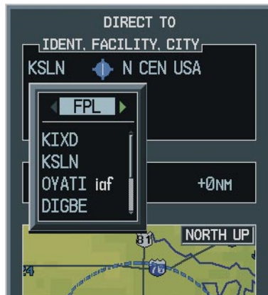
Figure 5-31 Flight Plan Waypoint List (MFD)
