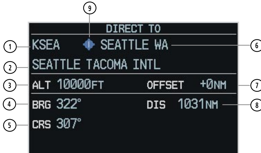
Figure 5-34 PFD Direct-to Window
