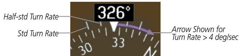
Figure 2-19 Turn Rate Indicator and Trend Vector
