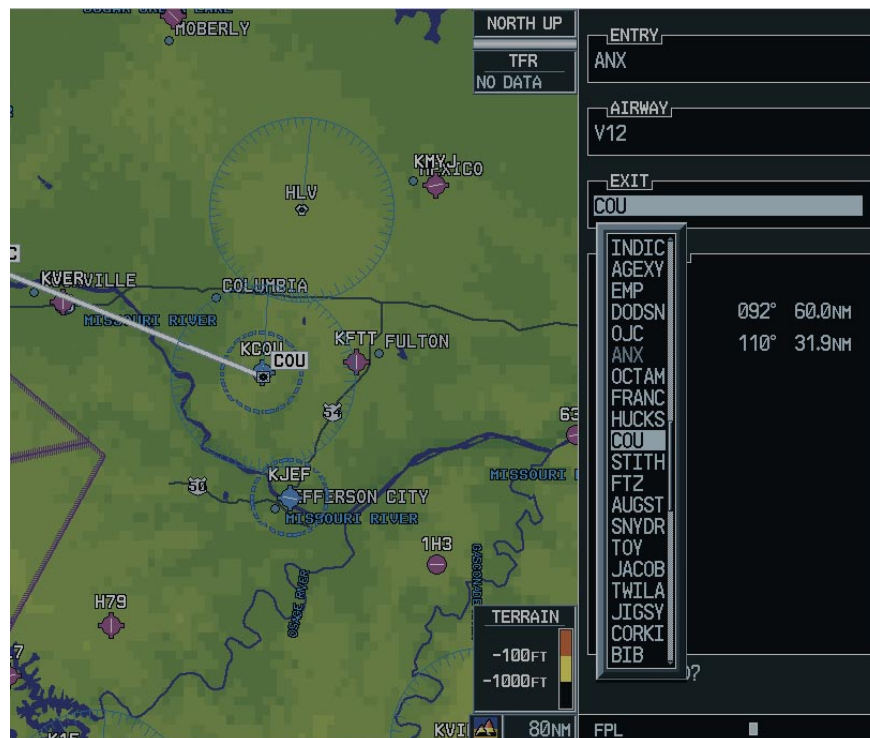
Figure 5-77 Selecting an Exit Waypoint
