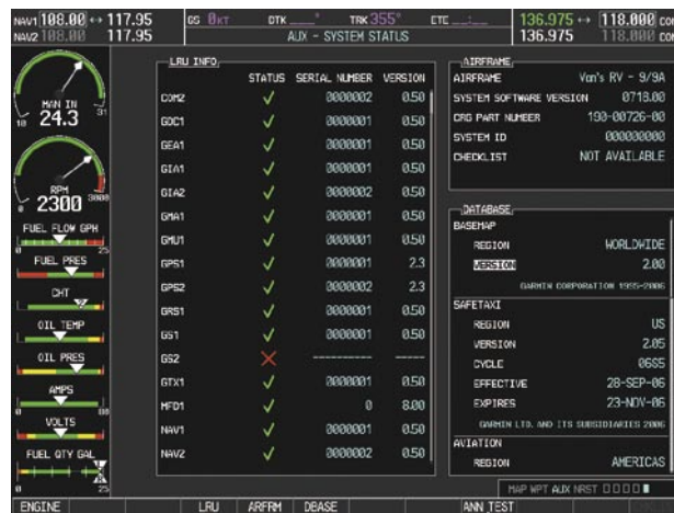
Figure A-2 System Status Page, Annunciation Tone Testing
