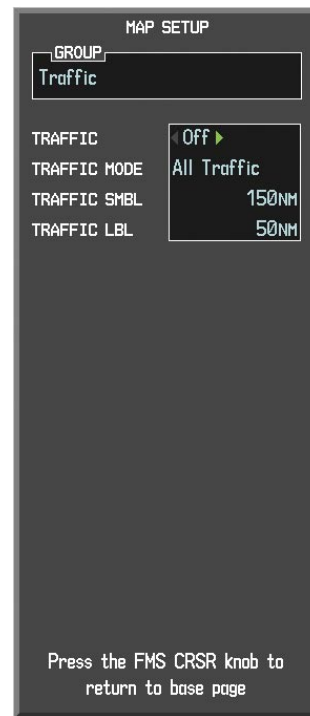
Figure 6-73 Navigation Map Page Setup Menu, Traffic Group
