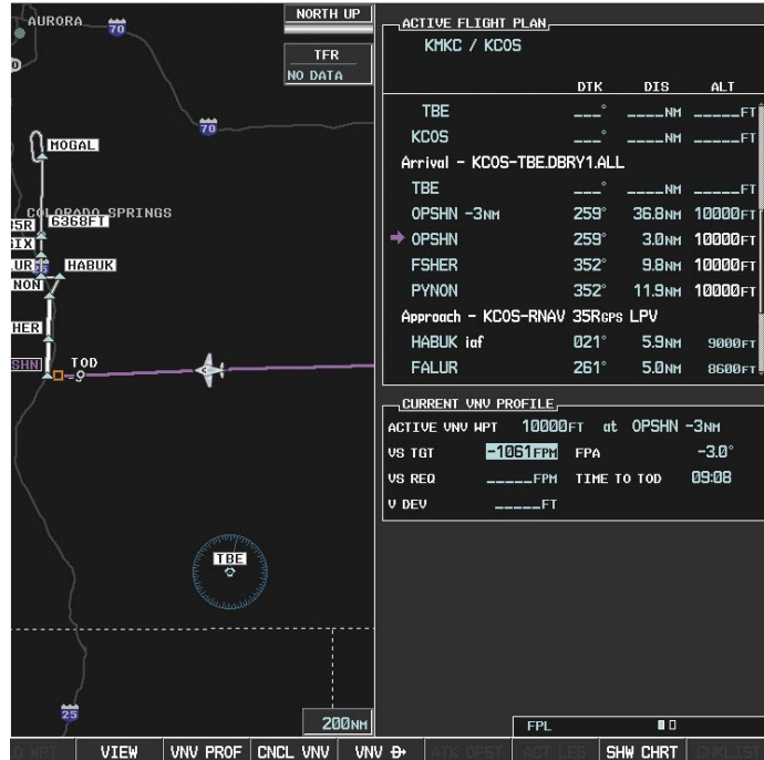
Figure 5-117 Adjusting the Descent
