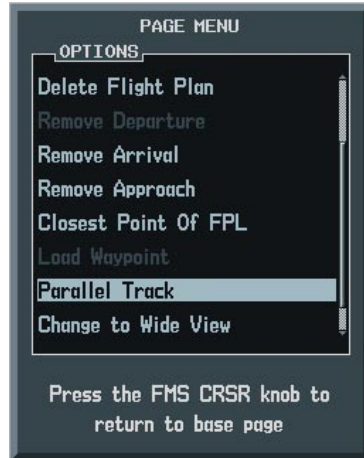
Figure 5-134 Parallel Track Menu Option
