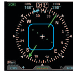
Figure 4-65 No Course Deviation Bar or TO/FROM Indicator
