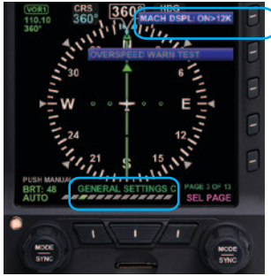
Figure 4-13a Altitude Transition Setting
