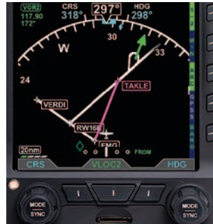
Figure 4-47 ARC CDI Compass Mode
