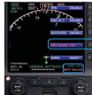
Figure 4-45 ARC CDI Compass MODE Selected
