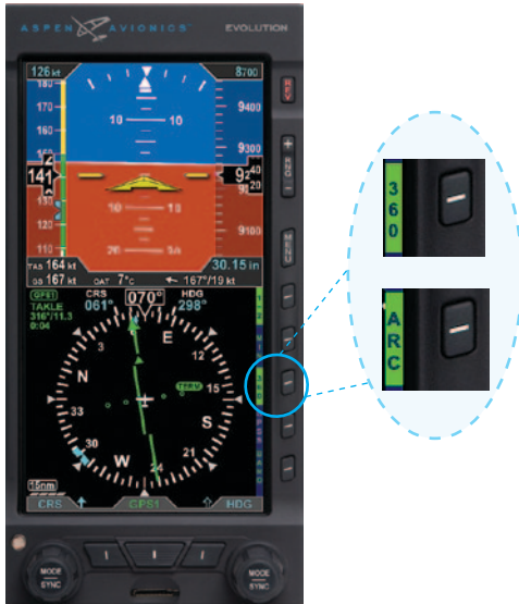
Figure 4-46 360/ARC Hot Key
