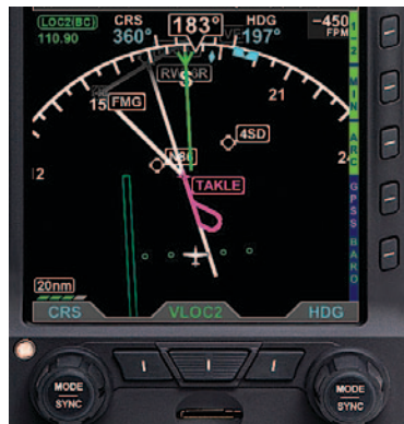
Figure 2-37 ARC CDI Compass Mode with Basemap
