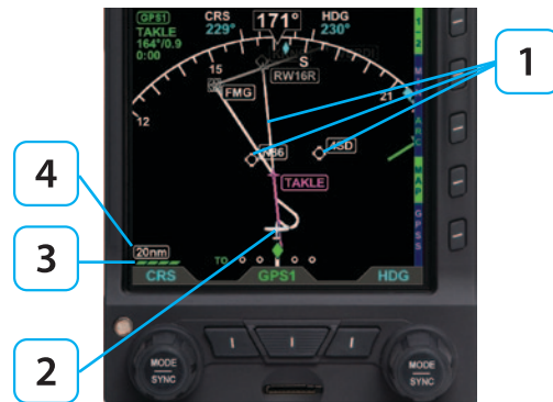
Figure 4-89 Basemap (ARC CDI Compass Mode Shown)
