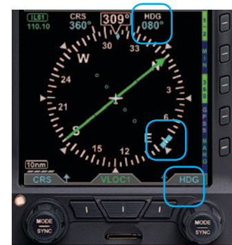
Figure 3-9 Selected Heading Field Disabled
