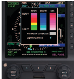
Figure 4-125 Data Link Weather Legend
