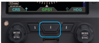
Figure 3-10 CDI Navigation Source Selection Button
