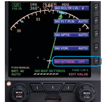
Figure 5-15 360° NDB Display Option Set To OFF
