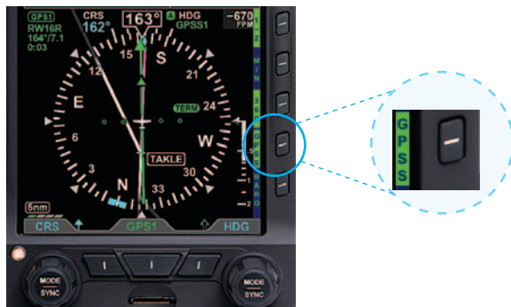
Figure 4-109 GPSS Hot Key
