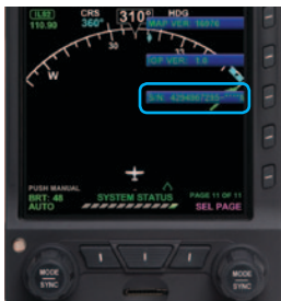
Figure 7-3 View Unit Serial Number
