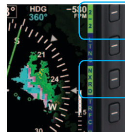
Figure 4-123 Data Link Weather Enabled
