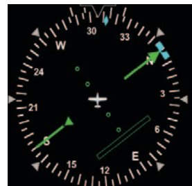
Figure 2-41 Off Scale CDI Bar
