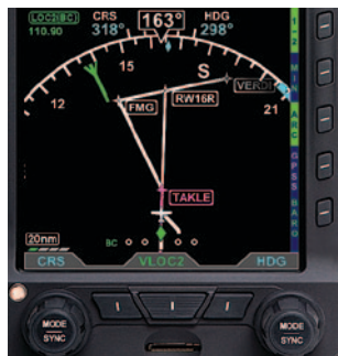
Figure 4-42 ARC CDI Compass Mode
