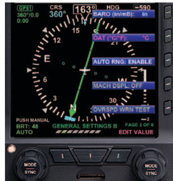
Figure 4-37 Select OAT Units of Measure
