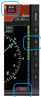
Figure 3-38 MIN Display Selected for Editing
