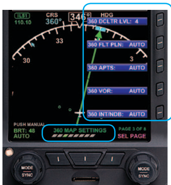
Figure 5-12 360° Compass Mode Display Options
