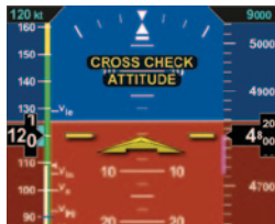
Figure 6-18 Cross Check Attitude
