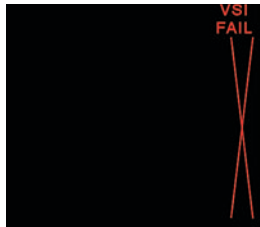
Figure 4-108 VSI Fail – 360° Compass Mode
