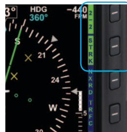
Figure 4-122 Lightning Overlay Enabled Displaying WX-500 Strike Data
