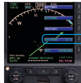
Figure 6-3 External Power Voltage Status
