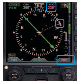
Figure 4-84 Heading Selected to Edit
