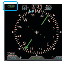
Figure 4-67 CDI Source Information Blank Block
