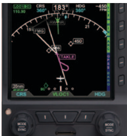
Figure 3-33 ARC CDI Compass Mode
