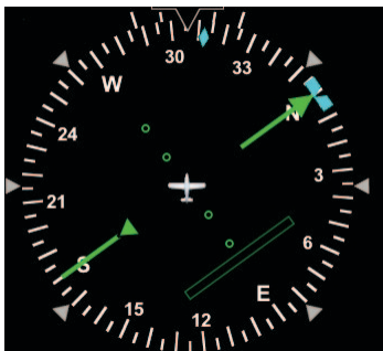
Figure 3-28 CDI Shown Hollow at Full-Scale Deflection
