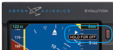
Figure 6-1 Powering Off the PFD
