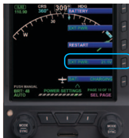
Figure 6-3 External Power Voltage Status
