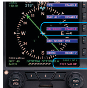
Figure 2-23 EDIT VALUE Displays Above Right Knob
