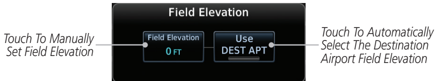
Figure 9-24 TCAD Traffic Field Elevation Selection
