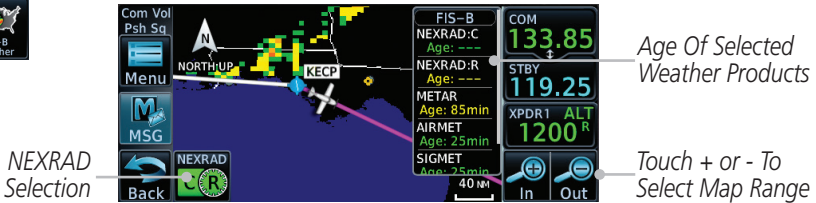
Figure 11-75 FIS-B Weather Page (NEXRAD Key Shown)
