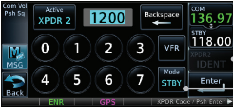
Figure 2-7 Transponder Mode "Standby" Indication
