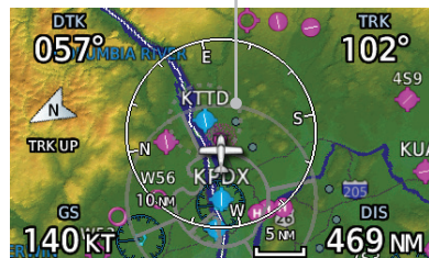
Figure 8-27 Display of Smart Airspaces (Airspace Borders Grayed)
