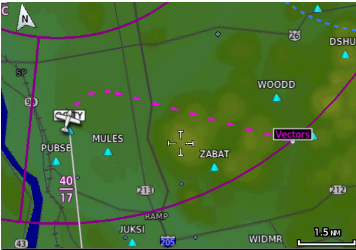
Figure 8-56 Active Heading Leg (Vectors)
