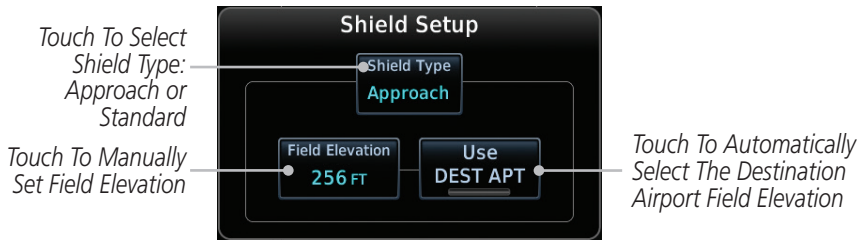
Figure 9-28 TCAD 9900B Shield Setup for Approach
