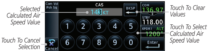
Figure 14-43 Select Calculated Air Speed Value
