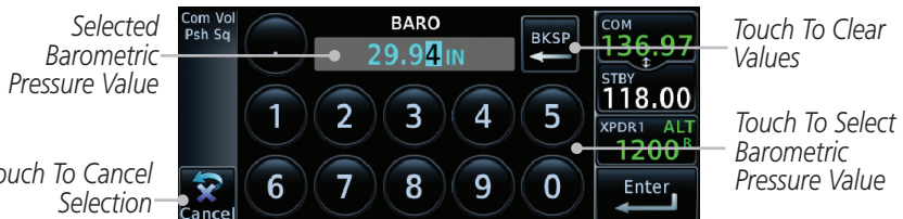
Figure 14-42 Select Barometric Pressure Value
