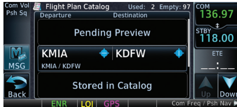
Figure 4-66 Catalog for Multiple Flight Plan Import
