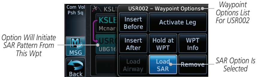
Figure 4-28 Active Flight Plan with Load SAR Option
