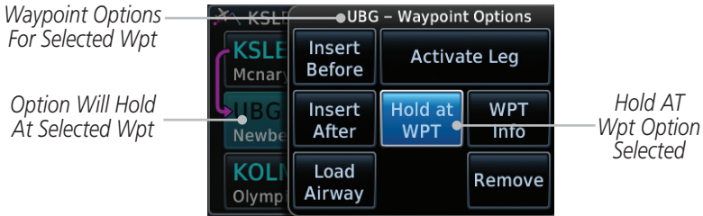
Figure 4-26 Active Flight Plan with Hold At Waypoint Option
