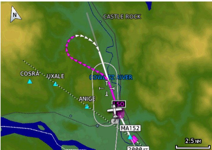
Figure 8-54 Active Procedure Turn
