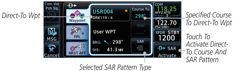
Figure 5-17 Direct-To Page with SAR Pattern Selected
