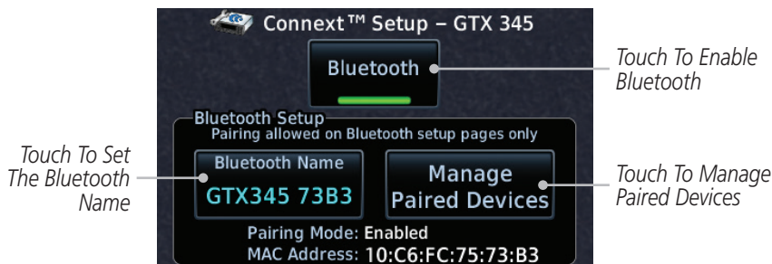
Figure 15-57 Connex Setup for GTX 345
