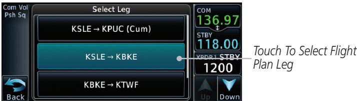
Figure 14-35 Select Flight Plan Leg
