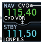
Figure 3-29 Automatic Nav Frequency Ident Decoding
