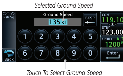
Figure 14-20 Selecting Expected Average Ground Speed
