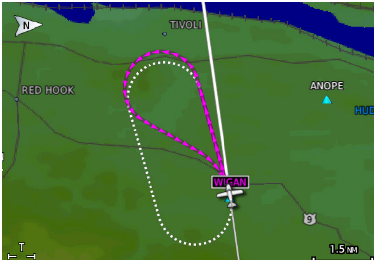
Figure 8-50 Holding Pattern Entry
