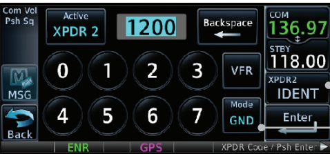
Figure 2-8 Transponder Mode "Ground" Indication
