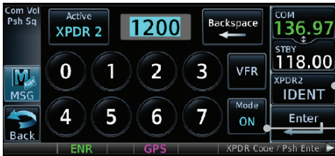
Figure 2-9 Transponder Mode "ON" Indication
