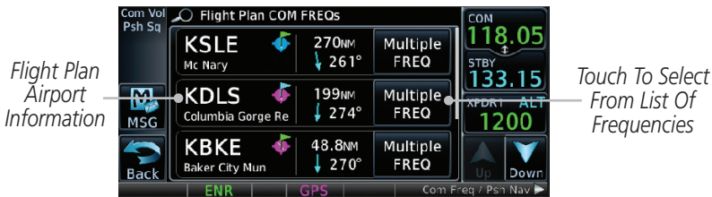
Figure 3-14 Flight Plan Frequency List
