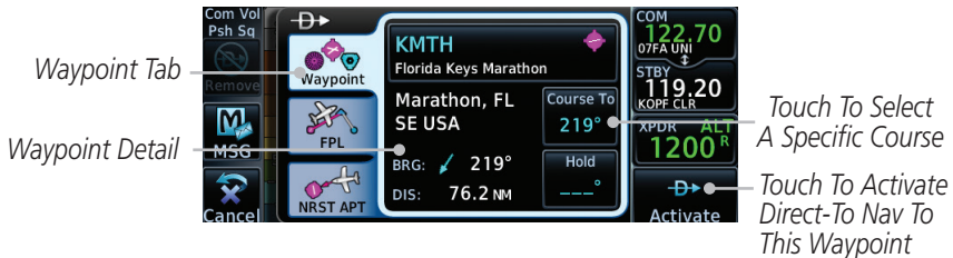
Figure 5-5 Selected Direct-To Flight Plan Leg
