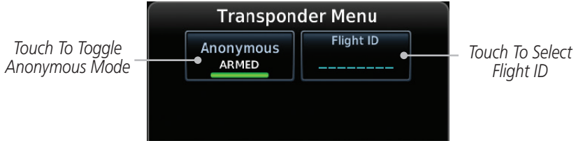
Figure 2-14 ADS-B/Transponder Control Panel
