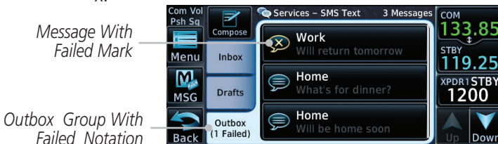
Figure 13-25 SMS Text Message List Showing a Failed Message
