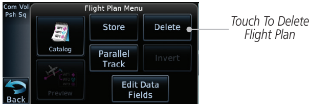
Figure 4-3 Delete Existing Flight Plan
