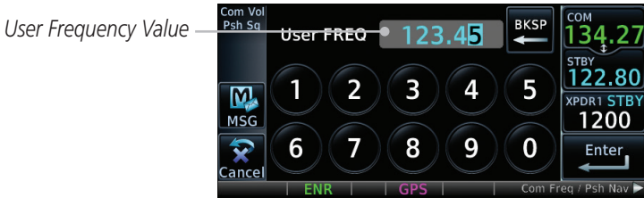
Figure 3-22 Select a Frequency Value for the New User Frequency
