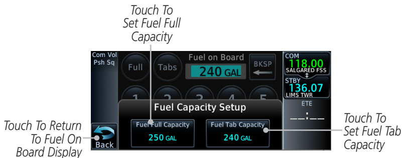
Figure 1-14 Fuel Capacity Setup Page
