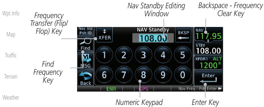
Figure 3-6 Nav Standby Frequency Numeric Keypad
