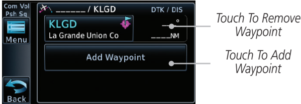
Figure 4-2 Create New Flight Plan
