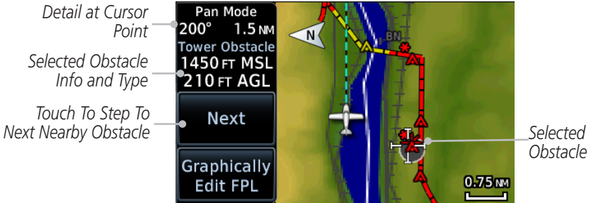
Figure 8-24 Point Obstacle Detail
