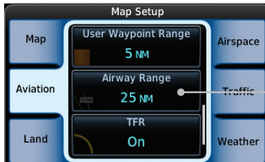
Figure 8-29 Map Setup For Airway Range
