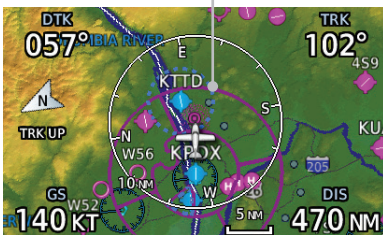
Figure 8-27 Display of Smart Airspaces (Airspace Borders Grayed)
