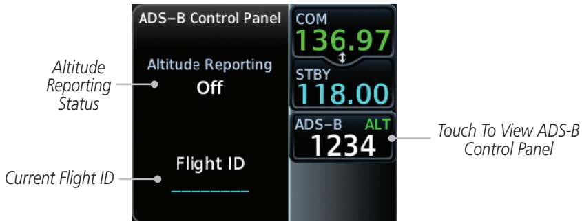
Figure 2-13 ADS-B Control Panel
