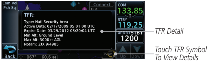
Figure 11-63 ConnexT TFR Detail
