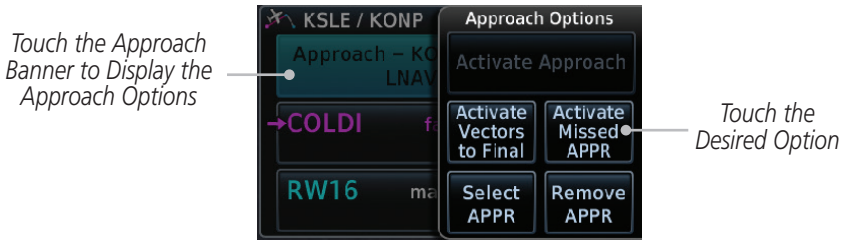
Figure 6-22 Approach Option Selection on the Flight Plan Page
