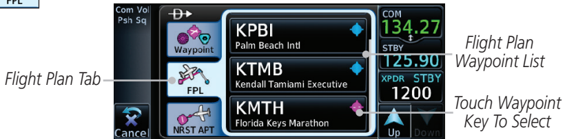
Figure 5-4 Direct-To Flight Plan Leg Selection
