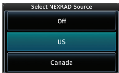
Figure 11-9 SiriusXM NEXRAD Weather Selection
