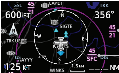
Figure 8-26 Display of Airspace Labels
