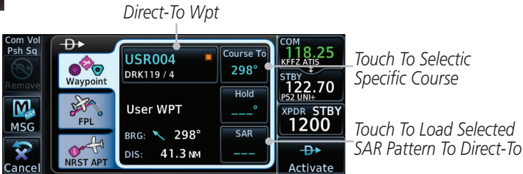
Figure 5-14 Create SAR Pattern at Direct-To Waypoint
