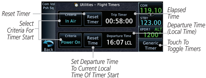
Figure 14-12 Utility Flight Timers Page (Trip/DEP Timers)
