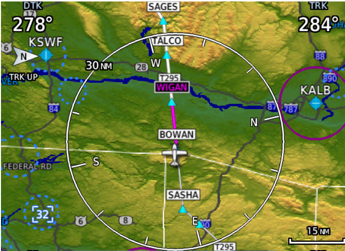
Figure 8-55 Past, Active, and Future Flight Plan Segments
