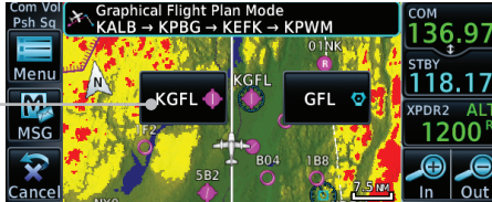
Figure 8-44 Select the Desired Waypoint From Multiple Waypoints
