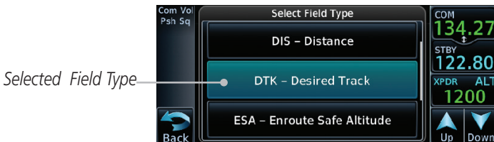
Figure 4-48 Flight Plan Data Fields List
