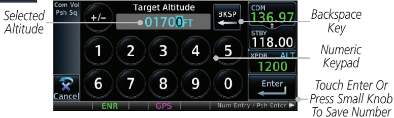
Figure 14-6 Select VCalc Target Altitude
