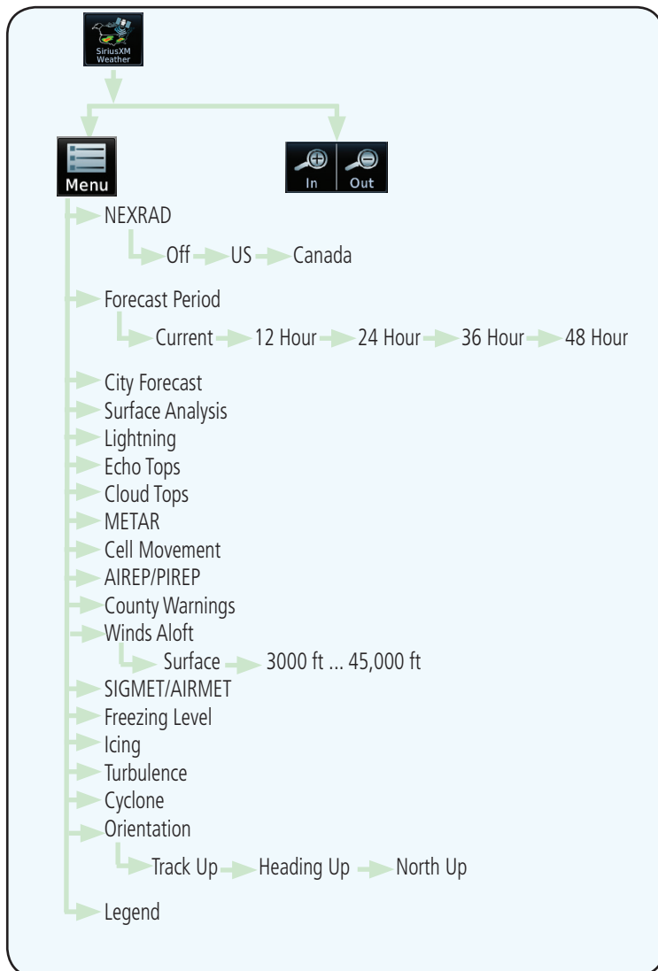
Figure 11-3 SiriusXM Weather Page Functional Diagram
