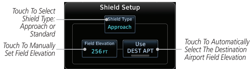
Figure 9-34 TCAD 9900BX Shield Setup for Approach
