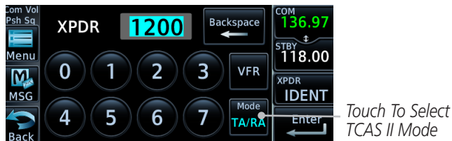
Figure 2-17 TCAS II Transponder Control Panel
