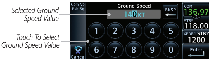
Figure 14-32 Selecting Ground Speed
