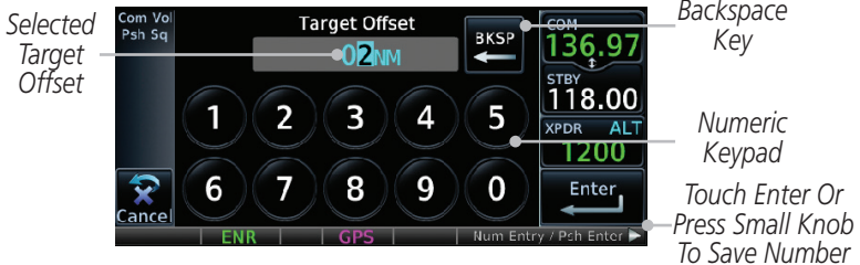
Figure 14-8 Select VCALC Target Offset
