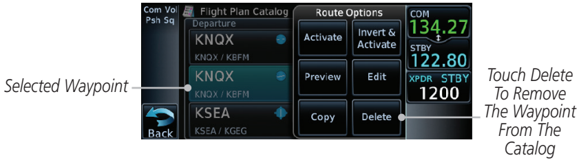
Figure 4-59 Select a Flight Plan from the Catalog
