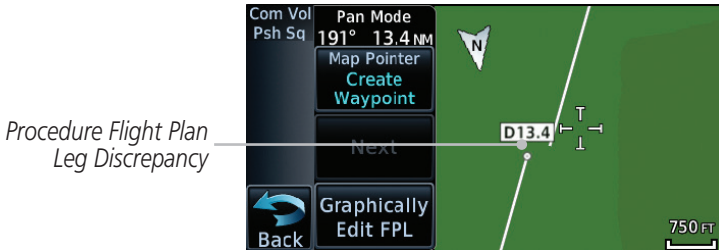
Figure 4-16 Procedure Flight Plan Leg Position Difference
